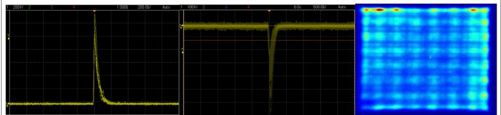
Figure 3. Outputs from the miniaturized analog front end. Left, transimpedance amplifier. Center, high bandwidth voltage feedback amplifier. Right first field flood image of intrinsic LYSO activity
