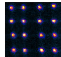
**Energy Resolution:** The energy spectra for each pixel was acquired. The mean FWHM for the 511keV photopeak obtained was 13.7%(figure 3). The spectrum corresponds to the active pixel area, depicted in blue on the figure.
