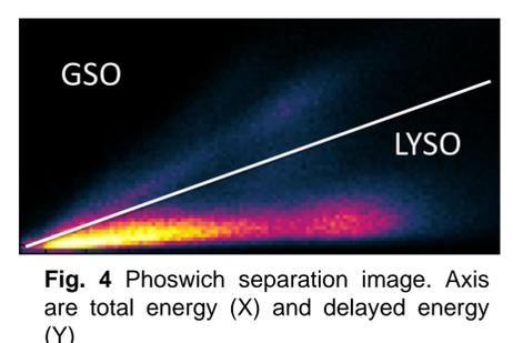
Fig. 4 Phoswich separation image. Axis are total energy (X) and delayed energy (Y)
