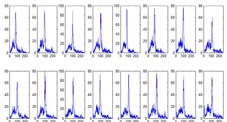
Fig. 3 Detector energy resolution measured on 16 pixels.
