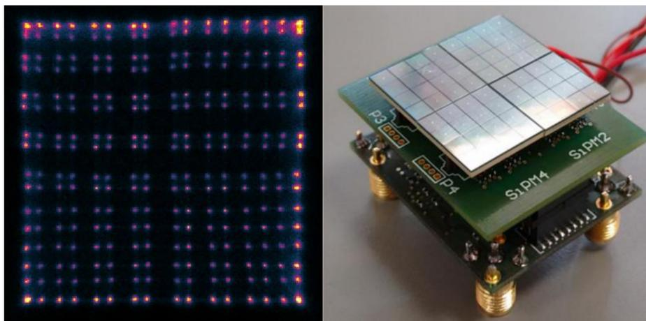
Fig. 1 Acquired image (without offset correction) and detector configuration used.
