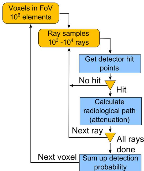
Fig. 2: Flowchart of sensitivity map algorithm.
