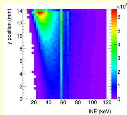
Figure 8. Number of interactions as a function of the depth in the detector ( $y = 14.08$  mm corresponds to the EOrow 255 and  $y = 0$  mm to the EOrow 0) and of the Initial Kinetic Energy of the incoming photon. It is clear, especially from the upper part, how the energy of the interacting photons increases with decreasing the EO row. This phenomenon, i.e. the energy discrimination, allows the spectral reconstruction to be performed.
