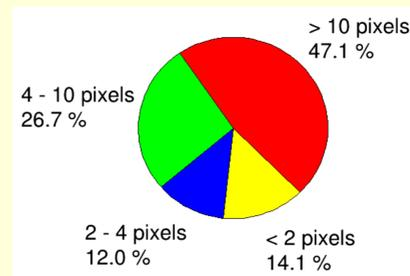
Figure 6. Distance (in pixel units) traveled by the scattered photon before it interacts again in the sensor. This interactions produce fake events.
