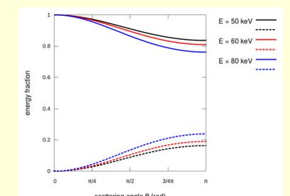
Figure 7. Energy fraction (energy transferred over energy of the incoming photon) deposited in a Compton scattering event for different energies of the incoming photon. The continuous line is for the scattered photon, the dashed one for the recoil electron.
