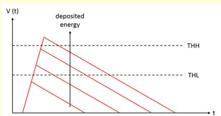
Figure 4. The charge produced by the incoming particle produces a triangular signal, which height is proportional to the energy deposited by the particle itself.
