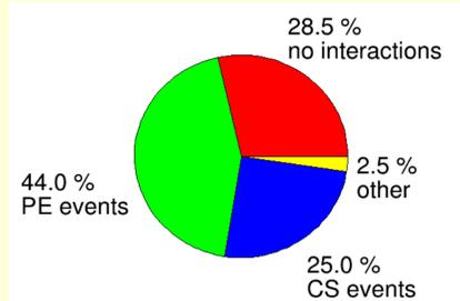
Figure 5. PE = PhotoElectric events (all the energy is deposited), CS = Compton Scattering events (the scattered photon escapes), other = photoelectrons that escape (1.7%) + Compton scattered photons that interact again in the sensor (0.8%)
