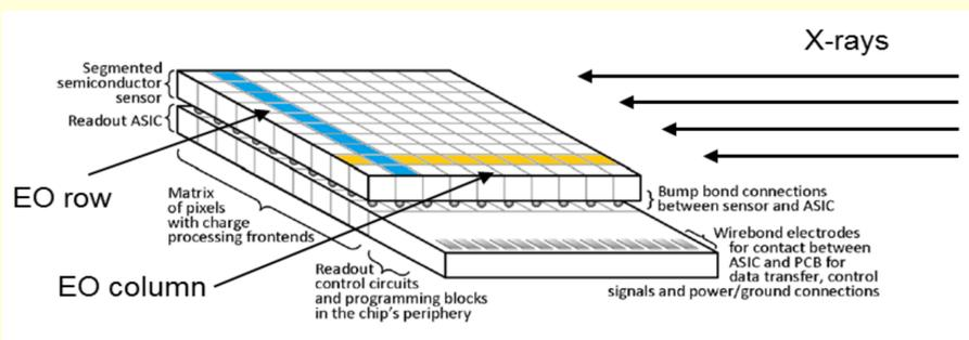
Figure 2. Schematic of the edge-on (EO) illumination. Usually the detector is used in face-on, with the X-rays coming from above, perpendicular to the detector matrix. Here the detector is rotated by 90°, with the X-rays impinging on the side of the sensor.
