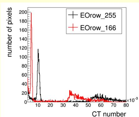
Figure 3. CT number histogram for two different EO rows; the peak from the same material appears translated. The CT number (or Hounsfield Unit) is a function of the energy of the photons, the density and the atomic number of the material. Since the two histograms belong to the same sample, the shift is due to the energy.
